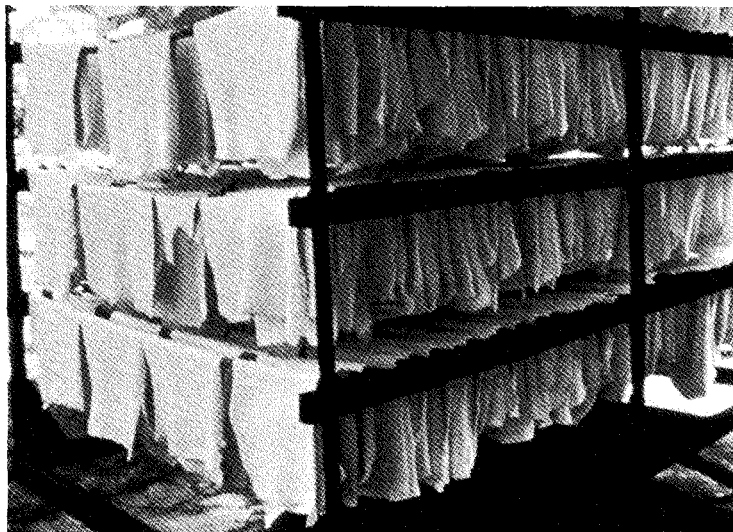
Rubber sheets hung on a trolley to be dried and smoked; they are compressed into bales for export. The growing global market for radial tires and other rubber products emphasizes the need to improve the quality of sheet that smallholders produce.
