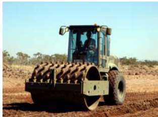
Compacted Clay Liner (CCL)
