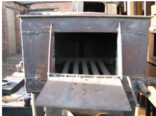
Low-Pressure Boiler Showing Water Pipes
