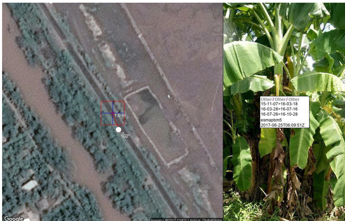
Figure 15: An example of a rejected reference field sample due to having been recorded in the middle of a road leaving uncertainty for the actual location of the field.
