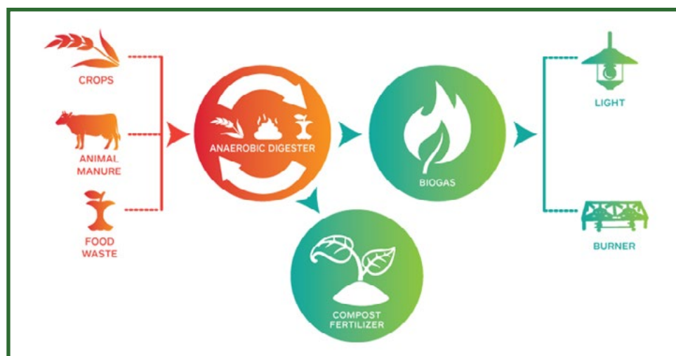
Figure 1. Schematic representation of a biogas digester
