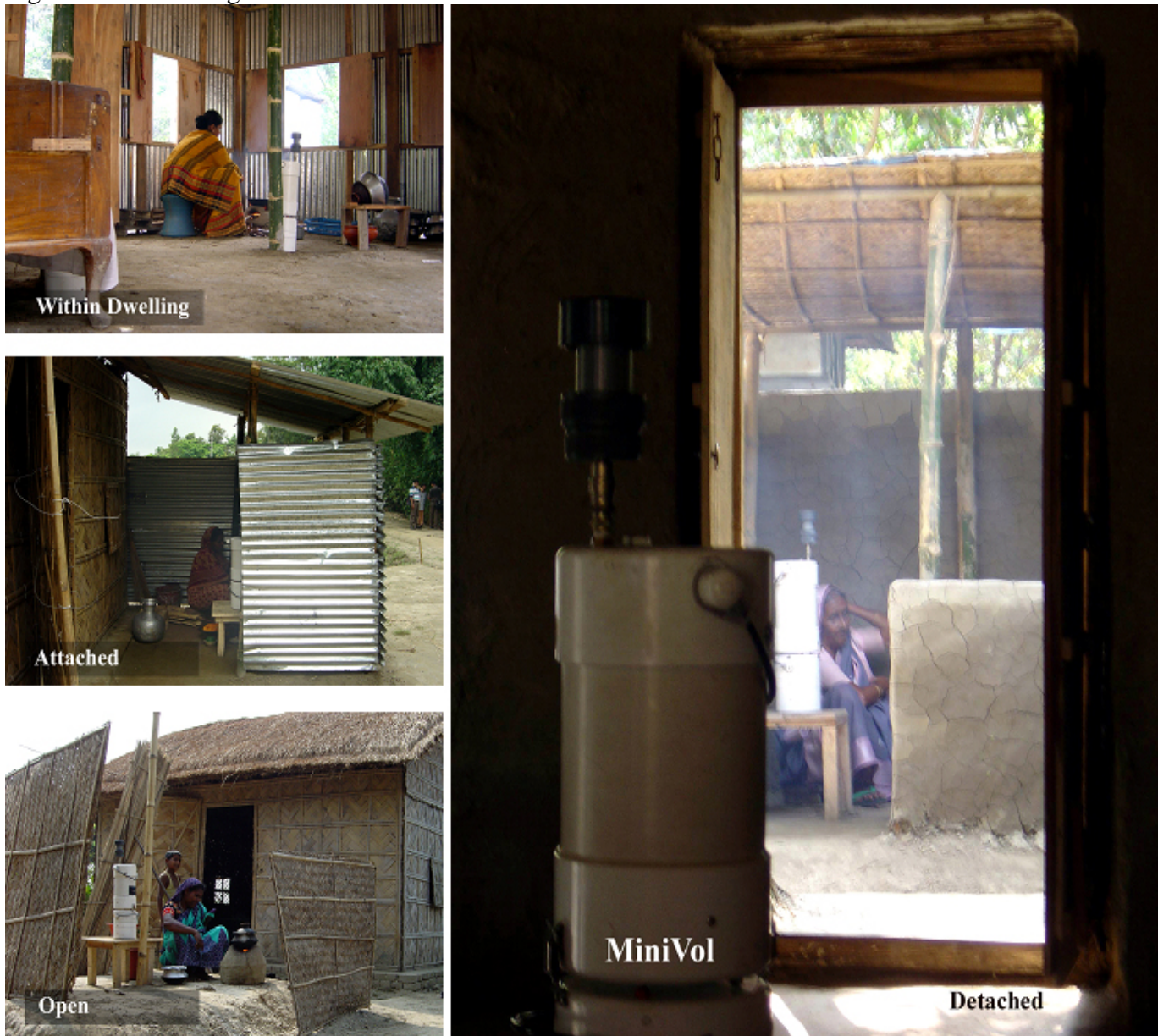
Figure 3: Monitoring Indoor Air in Different Kitchens
