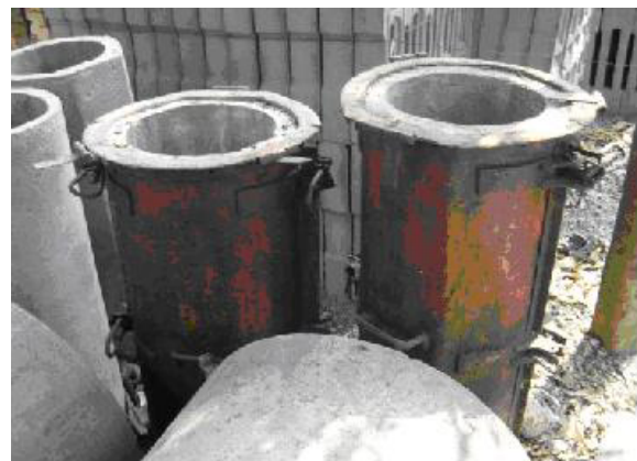
Steel rings to shape concrete, Lumajang district, January 2007
