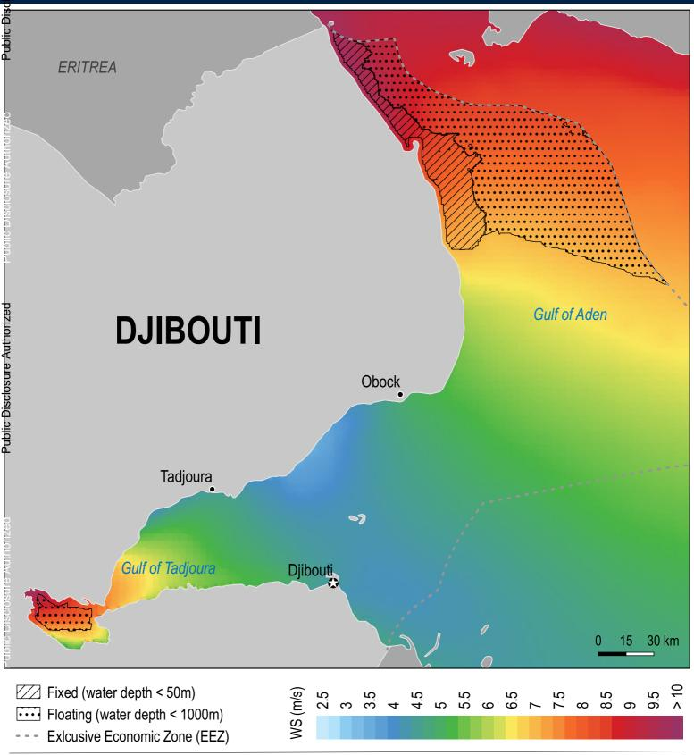
This map shows the estimated technical potential for fixed and floating offshore wind in Djibouti in terms of installed power capacity in megawatts (MW) within 200 kilometers of the shoreline. It is provided under a World Bank Group (WBG) initiative on offshore wind that is funded and led by the Energy Sector Management Assistance Program (ESMAP). For more information and to obtain maps for other WBG client countries please visit: https://esmap.org/offshore-wind.
