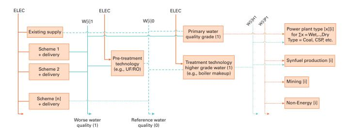
process is individually depicted, along with the required energy (electricity) inputs required to deliver the needed water. For a further explanation on how the regional WSCs were incorporated into SATIM-W, see appendix F.
