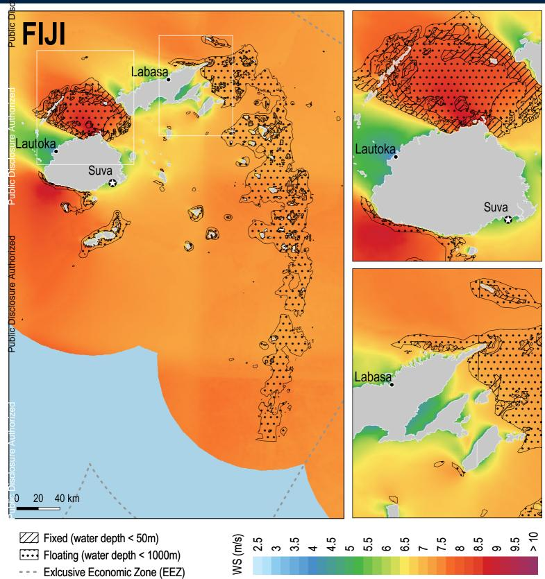
This map shows the estimated technical potential for fixed and floating offshore wind in Fiji in terms of installed power capacity in gigawatts (GW) within 200 kilometers of the shoreline. It is provided under a World Bank Group (WBG) initiative on offshore wind that is funded and led by the Energy Sector Management Assistance Program (ESMAP). For more information and to obtain maps for other WBG client countries please visit:
