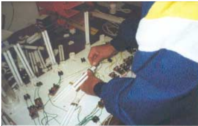
Figure 1.6 Assembly of a Compact Fluorescent Lamp in Botswana
