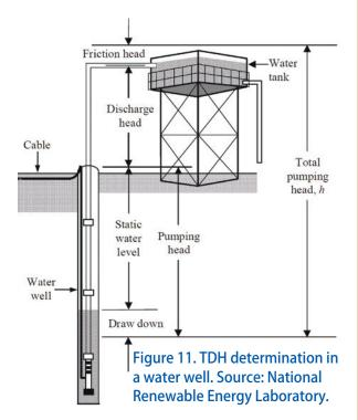
A pumping test can provide information on the DWL and the discharge head, whereas the friction head can be more accurately obtained from head loss charts for pipes at the required flow rate and pipe characteristics.
