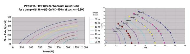
Figure 10. Pump motor characteristic P-Q curve and H-Q curve. Image credit: International Electrotechnical Commission, IEC.
