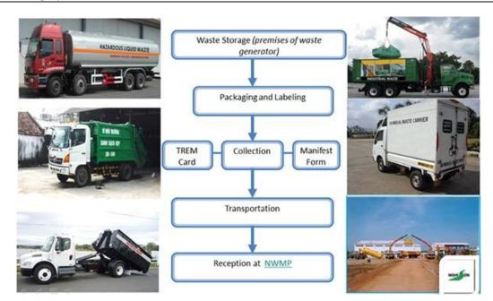
Figure 1. The process of collecting and transporting wastes to Nghi Son treatment plant
