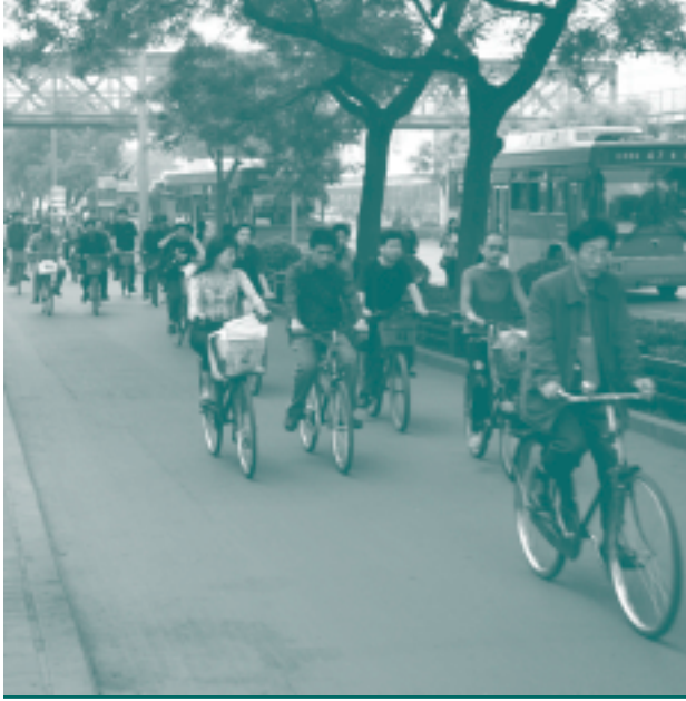
Segregating bicyclists from the rest of traffic, as this road in Beijing does, promotes nonmotorized transport, protects bicyclists' safety, and helps to keep traffic speed higher than when motorized and nonmotorized traffic are mixed.
